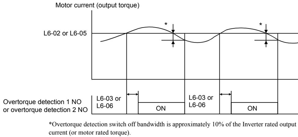
Fig 6.20 Overtorque Detection
