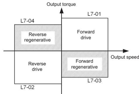
Fig 6.23 Torque Limit Parameters
