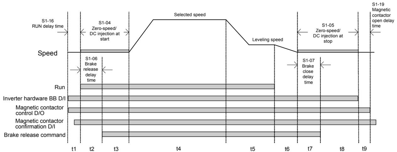
Fig 6.4 Timing Chart of Brake Sequence Without Torque Compensation at Start
