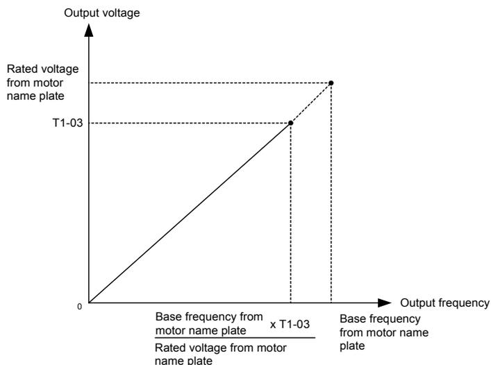
Fig 6.29 Motor Base Frequency and Inverter Input Voltage Setting
