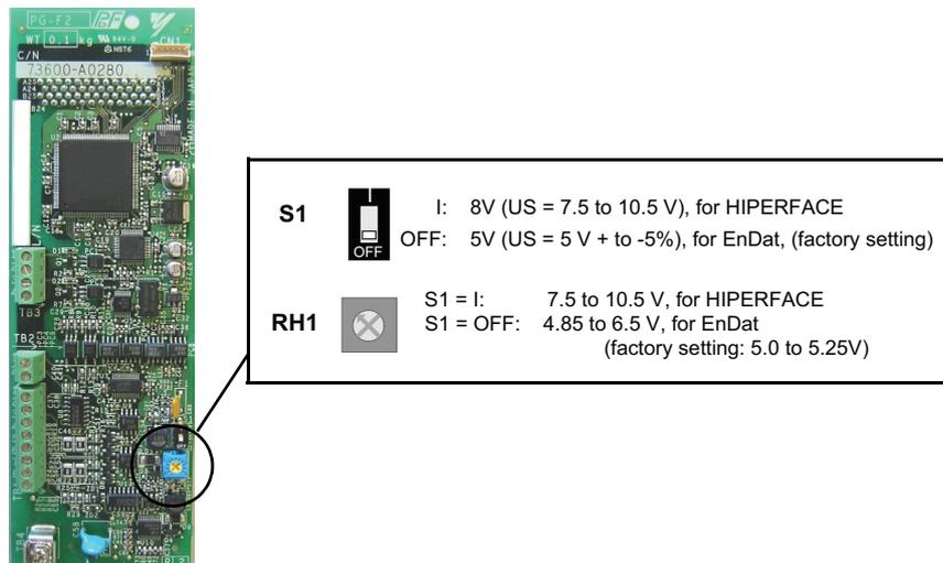
Fig 2.18 PG-F2 Encoder Power Supply Voltage Selection
