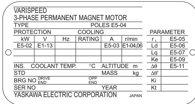
Fig 4.3 Nameplate Example for a Yaskawa permanent magnet motor
