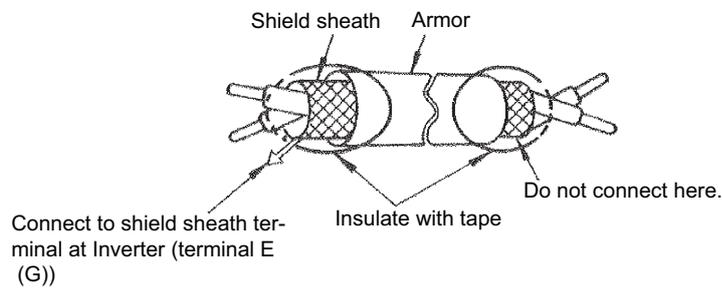
Fig 2.15 Processing the Ends of Shielded Twisted-pair Cables
