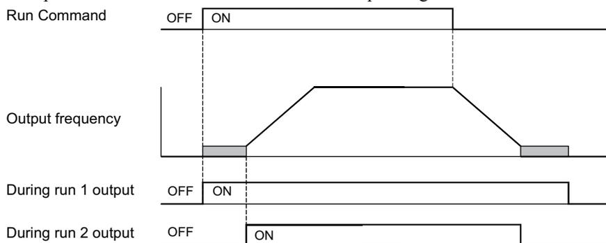
Fig 6.27 Timing Chart for "During RUN" Output
