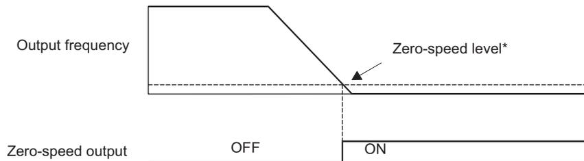
Fig 6.28 Timing Chart for Zero-speed
