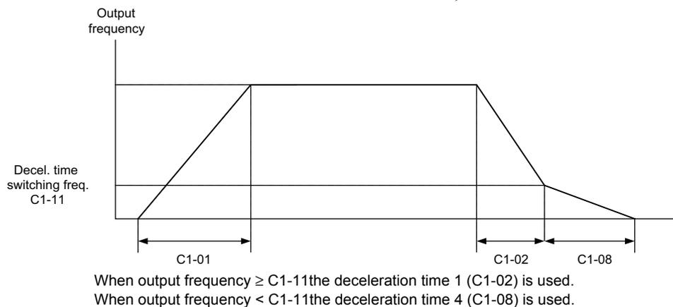
Fig 6.6 Acceleration/Deceleration Time Switching Frequency
