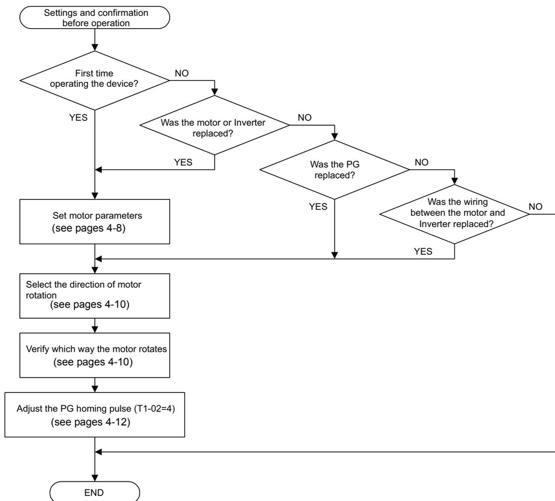
Fig 4.2 Settings and Data Verification Before Operating the Inverter
