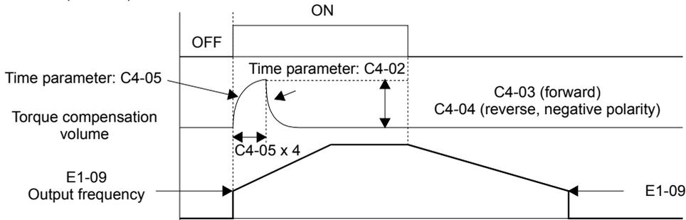
Fig 6.14 Time Chart for Starting Torque Frequency
