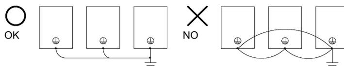
Fig 2.6 Ground Wiring
