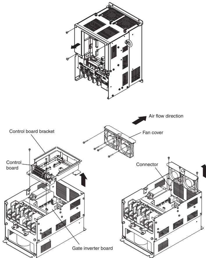
Fig 8.2 Cooling Fan Replacement (200 V Class Inverters of 22 kW)
