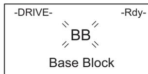
"BB Base Block" flashes on the Digital Operator screen.
