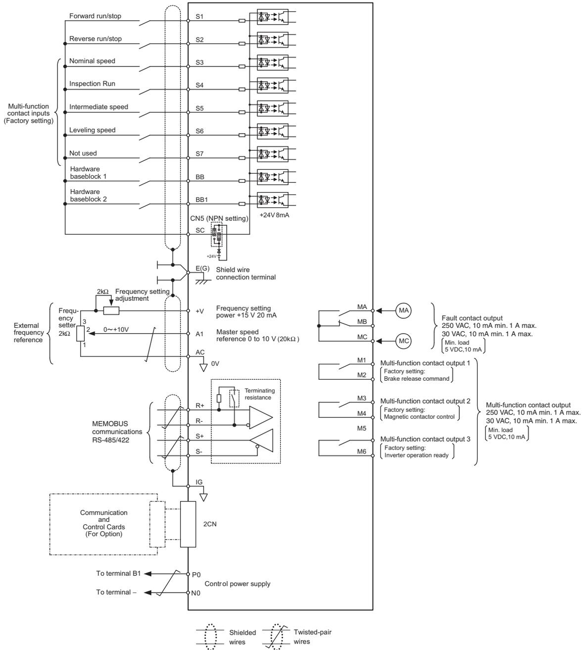
Fig 2.14 Control Circuit Terminal Connections
