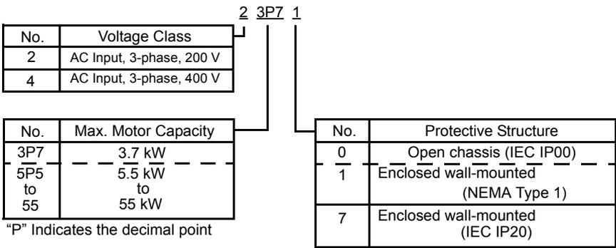
Fig 1.3 Inverter Specifications
