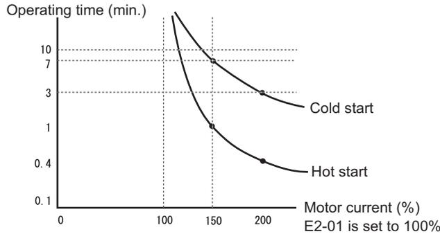
Fig 6.24 Motor Protection Operation Time
