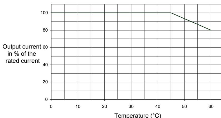
Fig 6.25 Ambient Temperature Derating Curve
