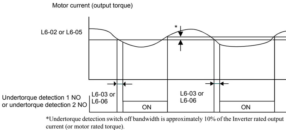
Fig 6.21 Undertorque Detection
