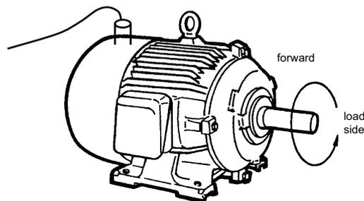
Fig 4.7 Direction of Motor Rotation
