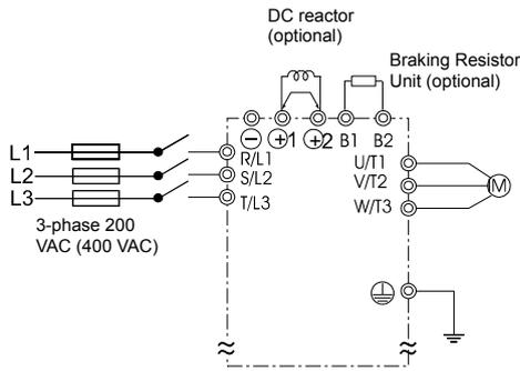
Be sure to remove the short-circuit bar before connecting the DC reactor.
