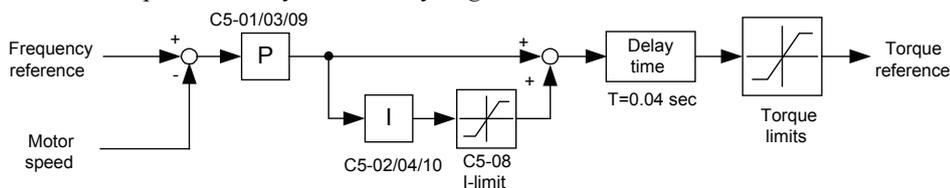
Fig 6.15 ASR Block Diagram
