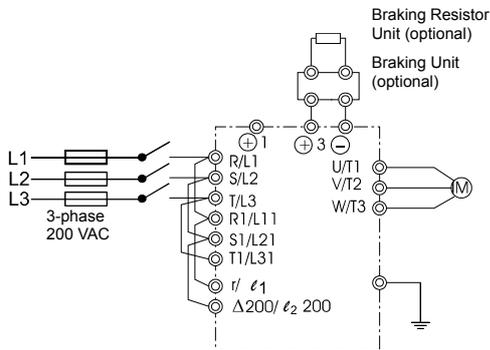
Control power is supplied internally from the DC bus at all Inverter models.
