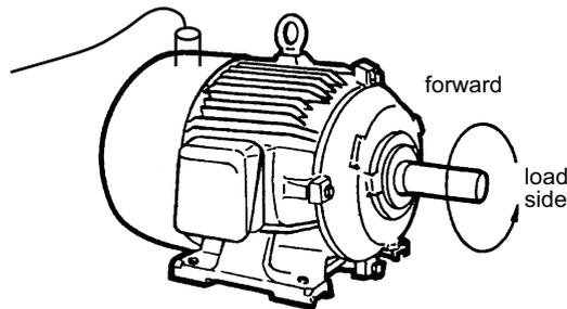
Fig 4.4 Direction of Motor Rotation
