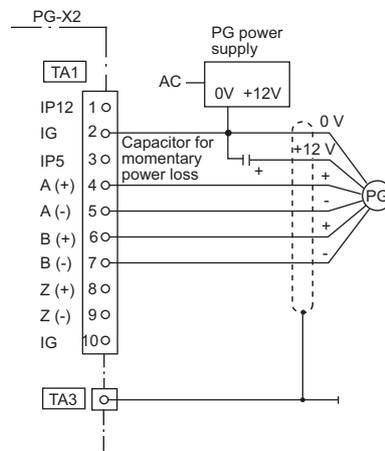
Fig 2.23 PG-X2 Connection Example (for 12 V PG power supply)
