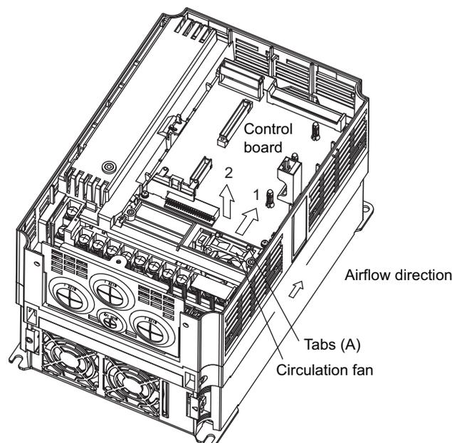
Inverter with Control Circuit Terminal Board Removed
