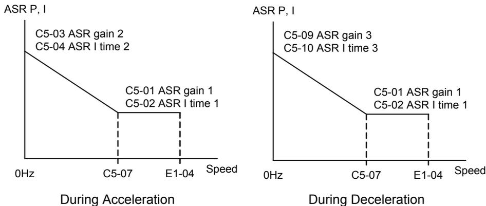
When the ride starts with the nominal speed selected, the ASR P gain and I time change from C5-03/04 to C1-01/02 at nominal speed. When the speed selection changes to leveling speed, the P gain and I time are changed from C1-01/02 to C1-09/10.
