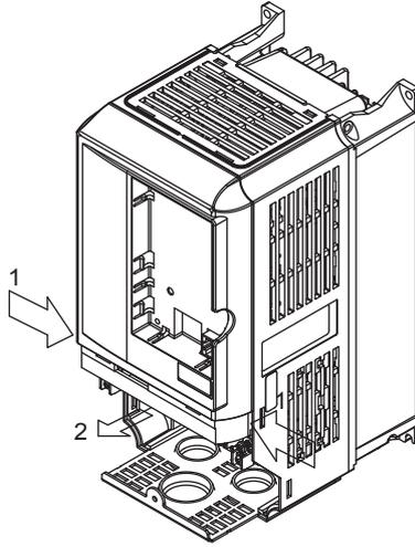
Fig 1.14 Removing the Front Cover (Model CIMR-L7B43P7 Shown Above)
