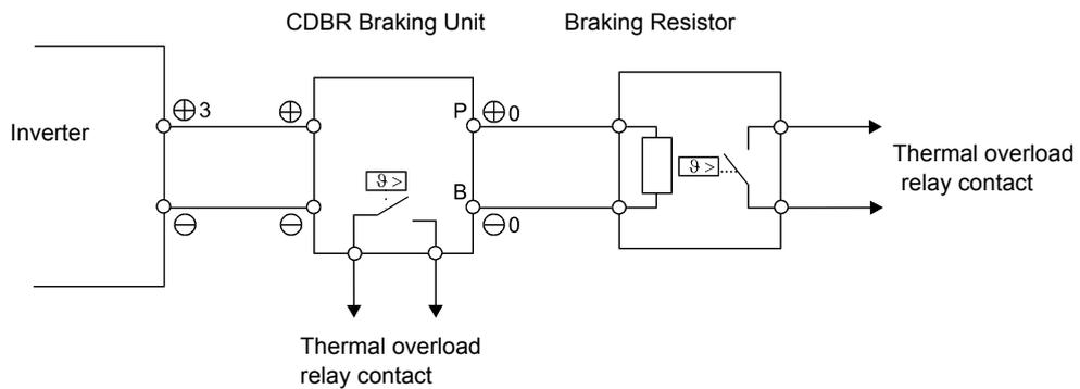
Fig 2.7 Connecting the Braking Resistor and Braking Unit
