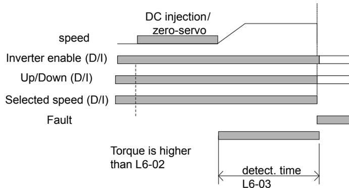
Fig 6.22 Car Stuck Fault Detection
