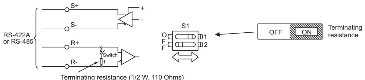
Fig 6.33 Communications Connection Terminal
