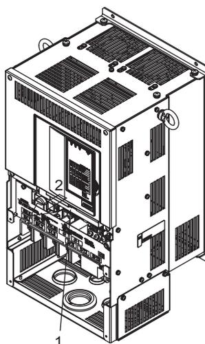
Fig 1.16 Removing the Front Cover (Model CIMR-L7B4022 Shown Above)
