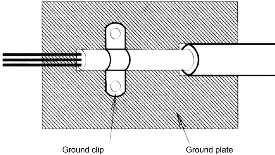
The grounding surfaces must be highly conductive bare metal. Remove any coats of varnish and paint.
