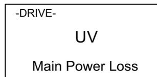
A fault or alarm message will appear on the display screen. The example shown here is for a low voltage alarm.
