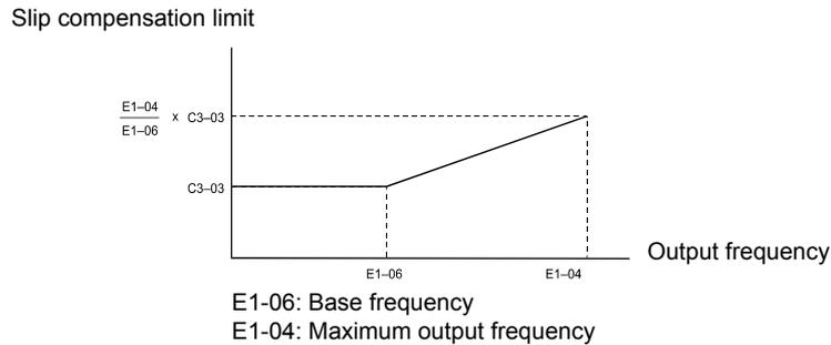
Fig 6.13 Slip Compensation Limit
