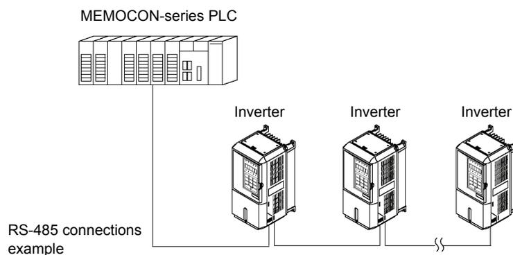
Fig 6.32 Example of Connections between PLC and Inverter
