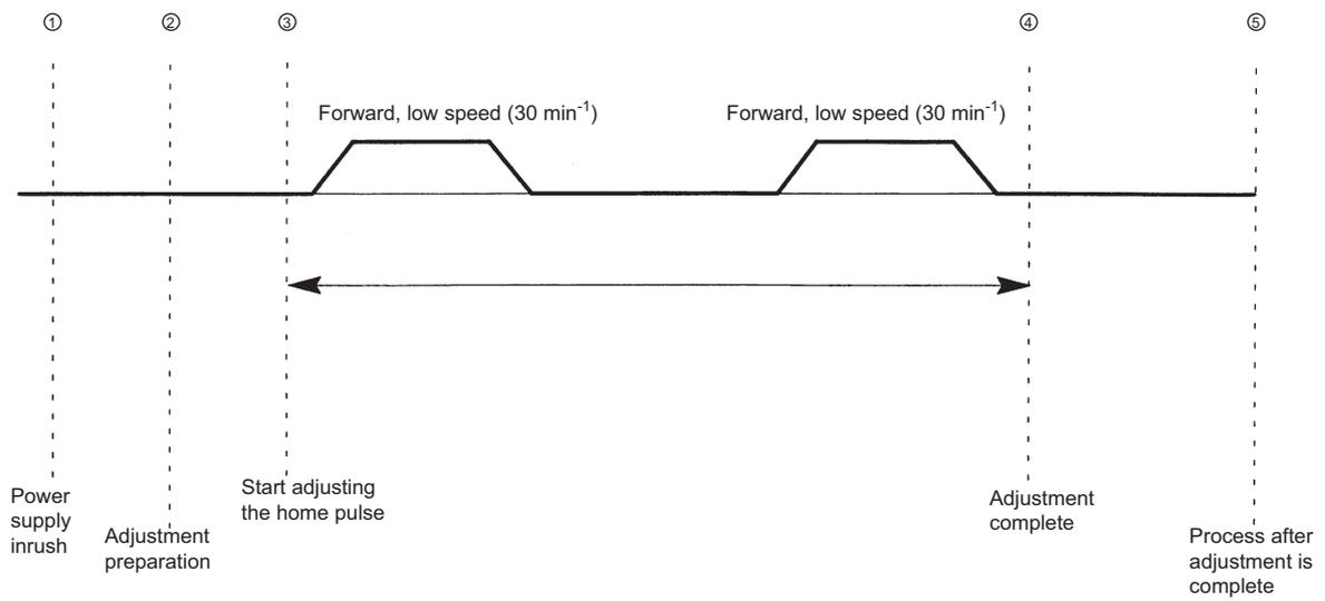
Fig 4.5 Adjusting the PG Home Location Pulse Offset, Pattern of Operation
