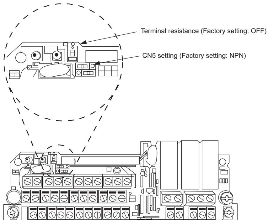
Fig 2.13 Shunt Connector CN5 and DIP Switch S1
