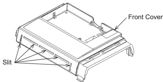
Fig 2.17 Cutting the Front Cover
