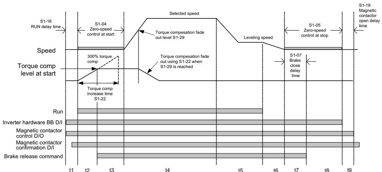
Fig 6.5 Timing Chart of Brake Sequence With Torque Compensation at Start
