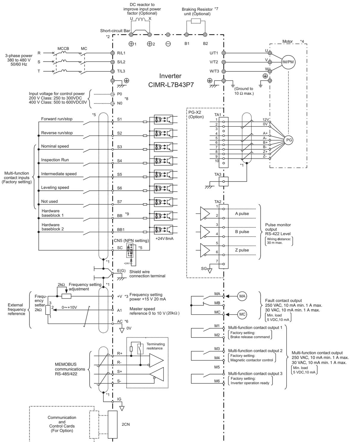
Fig 2.2 Connection Diagram (Model CIMR-L7B43P7 Shown Above)
