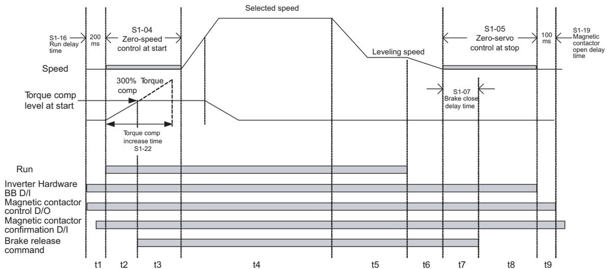
Fig 6.17 Timing Chart of Brake Sequence With Torque Compensation at Start
