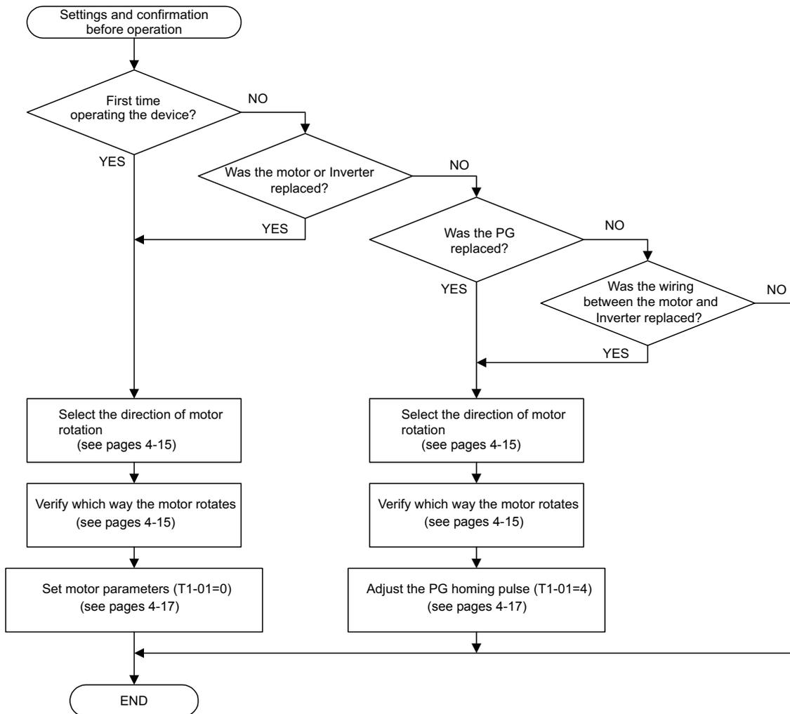
Fig 4.6 Settings and Data Verification Before Operating the Inverter
