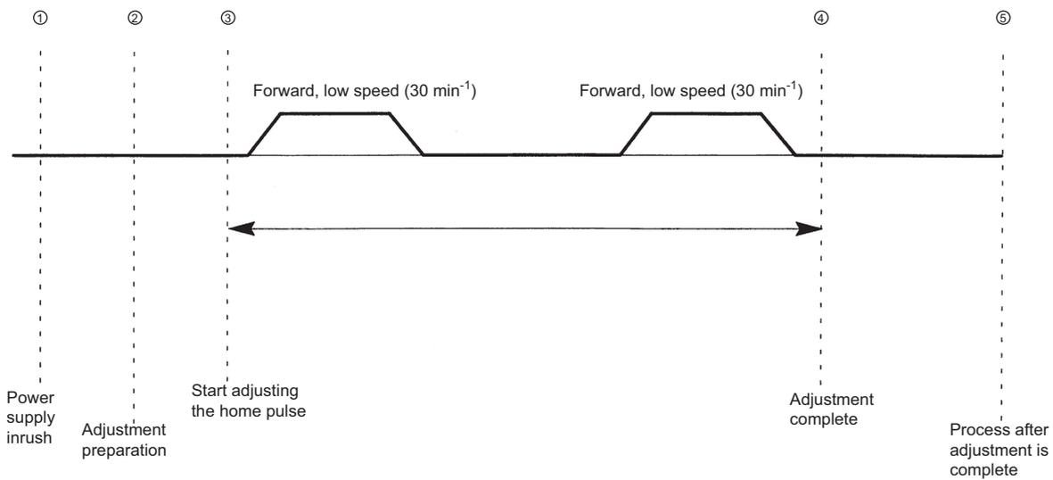
Fig 4.8 Adjusting the PG Home Location Pulse Offset, Pattern of Operation
