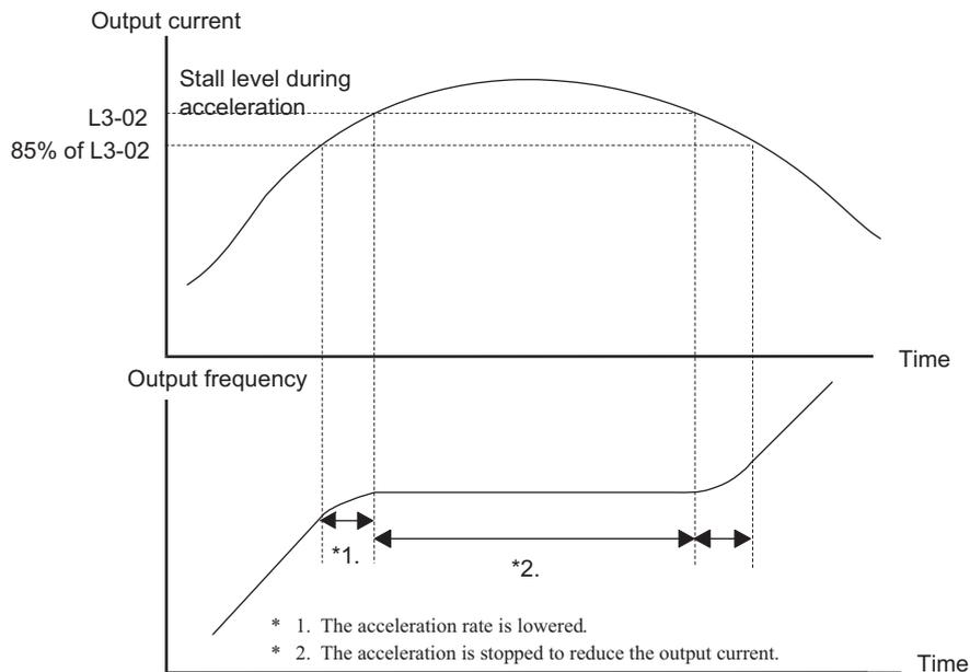
Fig 6.10 Time Chart for Stall Prevention During Acceleration
