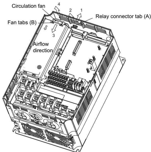
Fig 8.9 Circulation Fan Replacement (200 V and 400 V Class Inverters of 18.5 kW)
