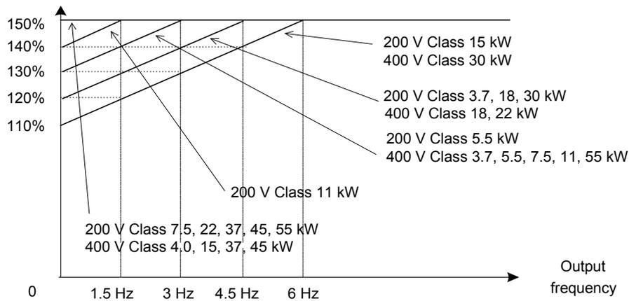
Fig 6.2 Low Frequency Current Limitation
