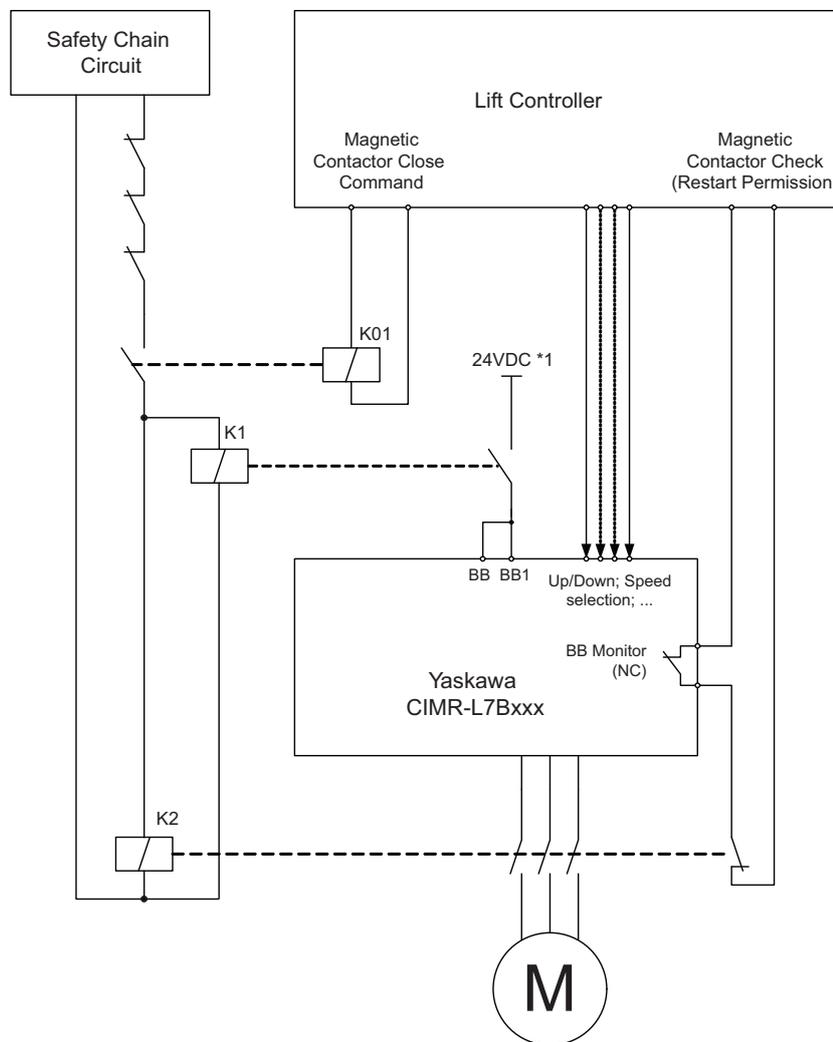
Fig 6.3 EN81-1 Conform Wiring with One Motor Magnetic Contactor (Example)
