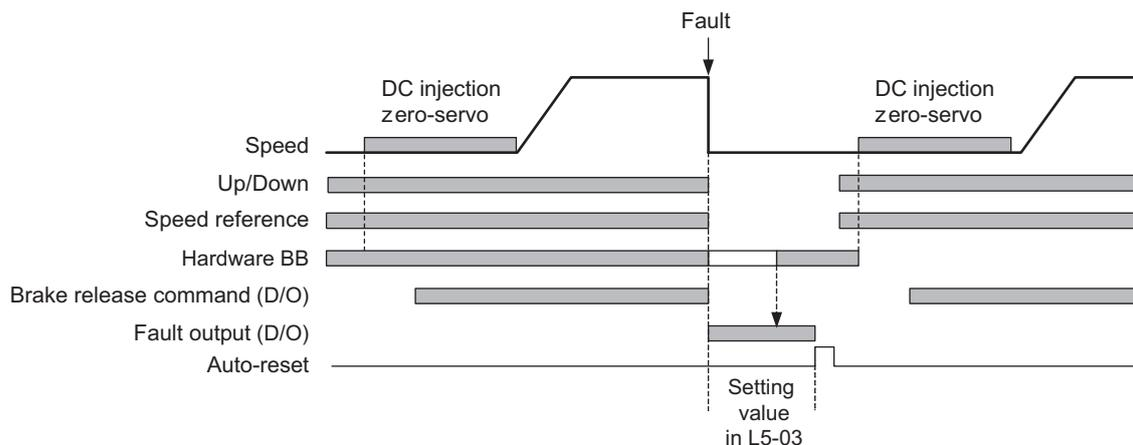
After receiving the hardware baseblock signal, the auto-reset signal can be received.
