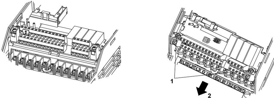
Fig 8.10 Removing the Control Circuit Terminal Board
