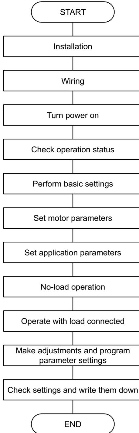
Fig 4.1 Trial Operation Flowchart
