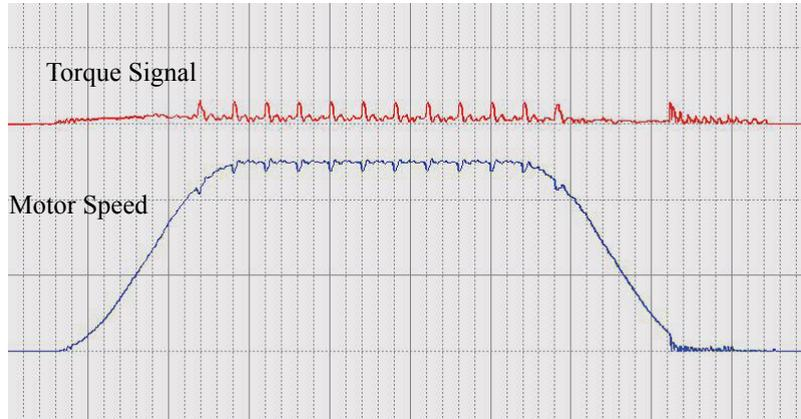
Fig 6.16 Oscillations Caused by Bad A/D Conversion Adjustment
