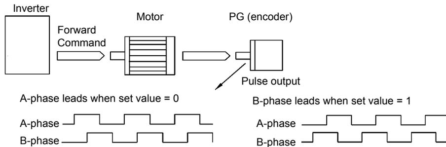
Example: Forward rotation of standard motor (PG)
