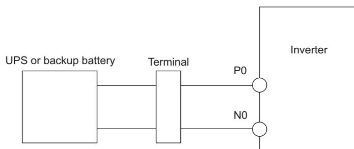
Fig 2.9 Connecting a Backup Battery
