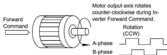
With the used PG the A-phase leads (CCW) when motor rotation is forward.
