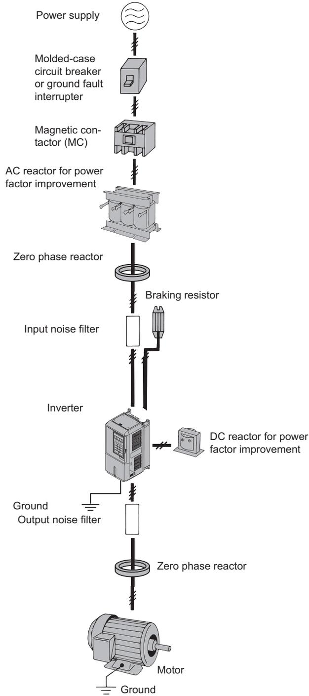
Fig 2.1 Example Connections to Peripheral Devices
