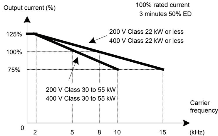
Fig 6.1 Current Rating Depending on the Carrier Frequency
