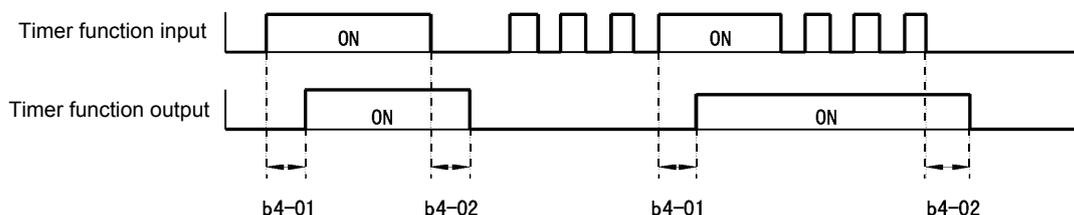
Fig 6.26 Timer Function Operation Example
