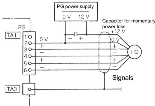
Fig 2.22 PG-B2 Connection Example
