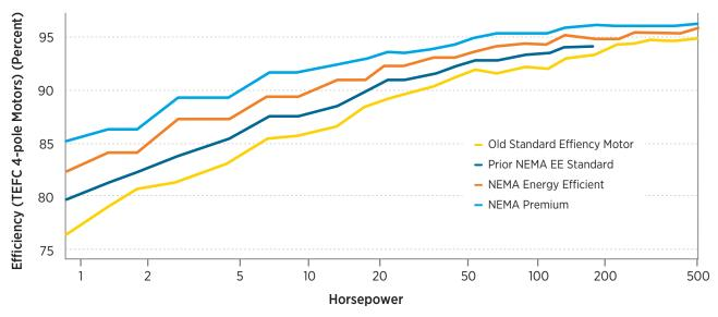
Figure 2-1. Standard, energy-efficient and premium efficiency motor performance
