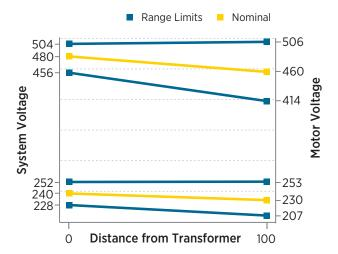
Figure 9-1. Acceptable motor utilization voltage range
