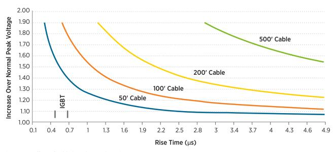
Figure 5-5. Effect of cable length on voltage increase. Source: John Fluke Manufacturing Company
