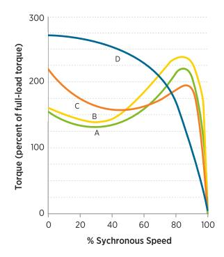
Figure 6-5. Typical speed/torque comparisons of NEMA design A-D induction motors
