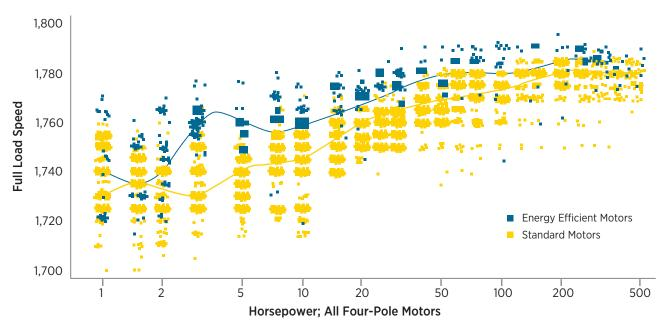
Figure 4-3. Full-load speed characteristics of standard and energy efficient motors
