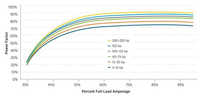
Figure 4-5. Motor power factor as a function of percent full-load amperage
