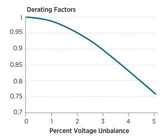
Figure 5-2. Motor derating due to voltage unbalance
