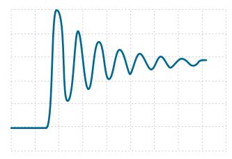
Figure 6-7. PWM pulse with reflected voltage or ringing
