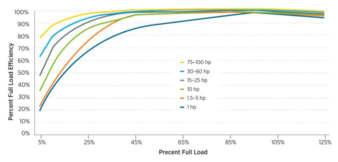
Figure 4-4. Motor part load efficiency as a function of percent full-load efficiency
