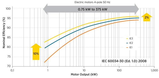
Figure 2-3. IEC motor efficiency classes
