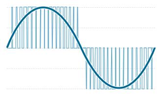
Figure 5-4. Sine wave overlaid on square carrier waves
