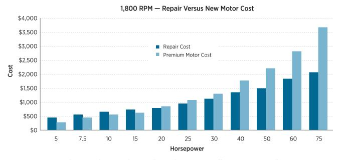
Figure 4-1. Motor repair (bearing replacement plus rewinding) and new premium efficiency motor costs (for 1,800 RPM TEFC motors, 2011 prices)
