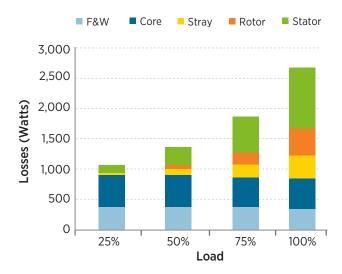
Figure 2-4. Losses versus Motor Load for a Standard **Efficiency Motor**
