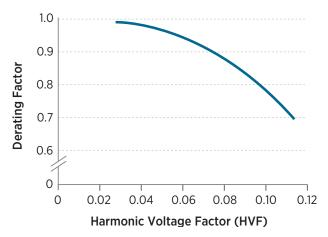
Figure 9-2. Harmonic voltage derating curve
