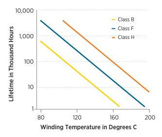
Figure 6-4. Service life versus operating temperature for motor insulation systems
