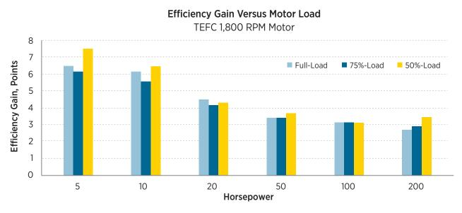
Figure 6-3. Efficiency improvement versus motor load (premium versus standard efficiency 1,800 RPM TEFC motors)
