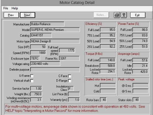
Figure 2-6. Typical MotorMaster+ motor database search results and motor detailed reports
